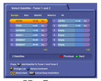
Press the A and buttons here to select the satellites you want tuners 1 and 2 to receive signals
